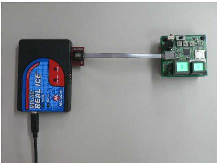
PICkit™ 2 + AC164110 - RJ-11 to ICSP Adapter, MPLAB REAL ICE, or others (Left photo shows MPLAB REAL ICE connected to the evaluation kit. )
